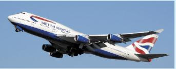
plant, at Everett in Washington state, was built to produce the huge aircraft with its 200ft wingspan, 8300 mile range and 550 mph cruising speed. To date 1400 Jumbos have been delivered, with a further 100 currently on order and a continuing development programme of future variants.
