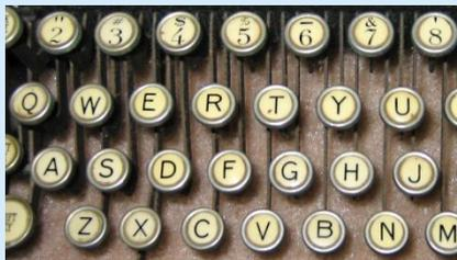
Devised in the 1870s, the familiar **QWERTY** keyboard layout was arranged in staggered columns to accommodate the operating levers of mechanical typewriters and with a key sequence designed to avoid clashes when typing at speed.
