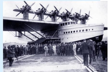
based in the machine centre deep in the hull, and who controlled the multiple throttles of its twelve engines (six pull + six push), to adjust power as necessary. Despite its luxurious passenger accommodation the aircraft was not a success...
